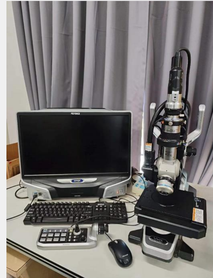
Figure 4 | Optical microscope system
